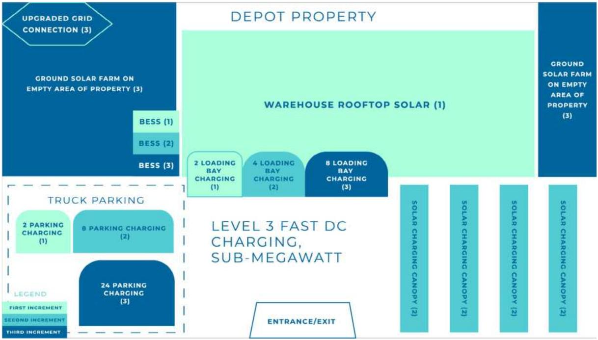
Figure 2: Simplified layout of increments of additional capacity
