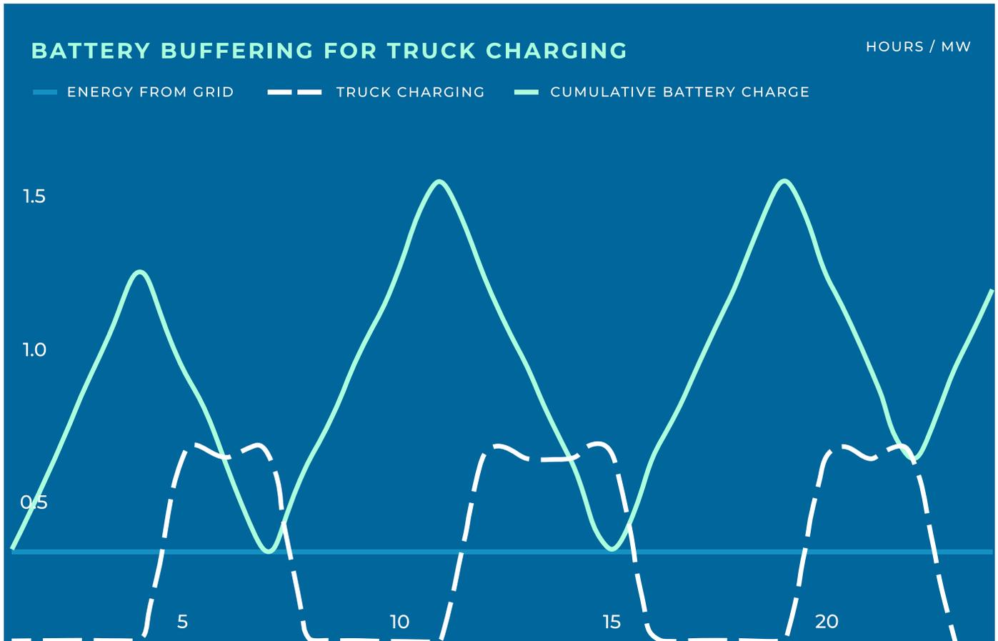
Figure 1: simple battery buffering pattern for low levels of trucks
