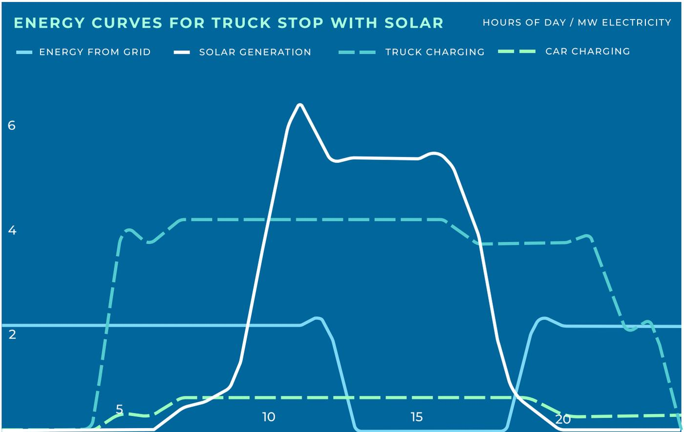
Figure 1: Electricity supply and demand curves for solar and battery microgrid truck stop
