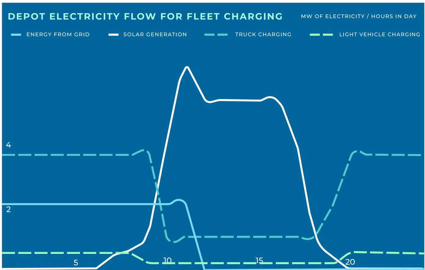
Figure 2: Electricity flows for charging trucks and light vehicles at depot
